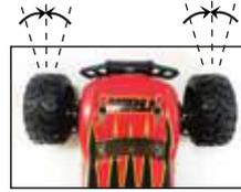
Left Knob. Used to set the steering neutral point on front wheels. If the front wheels on the vehicle veer in one direction while the steering wheel is centered, turn this knob in the opposite direction until the vehicle drives straight.
