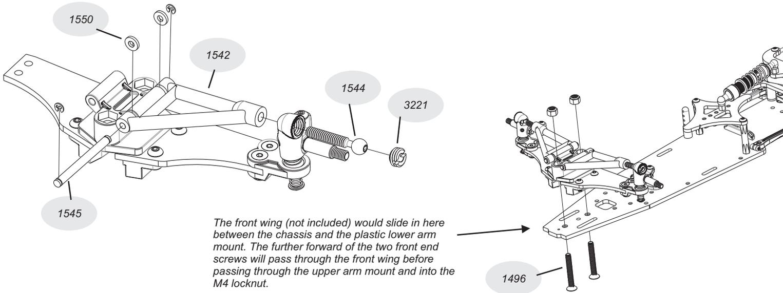
The front wing (not included) would slide in here between the chassis and the plastic lower arm mount. The further forward of the two front end screws will pass through the front wing before passing through the upper arm mount and into the M4 locknut.
