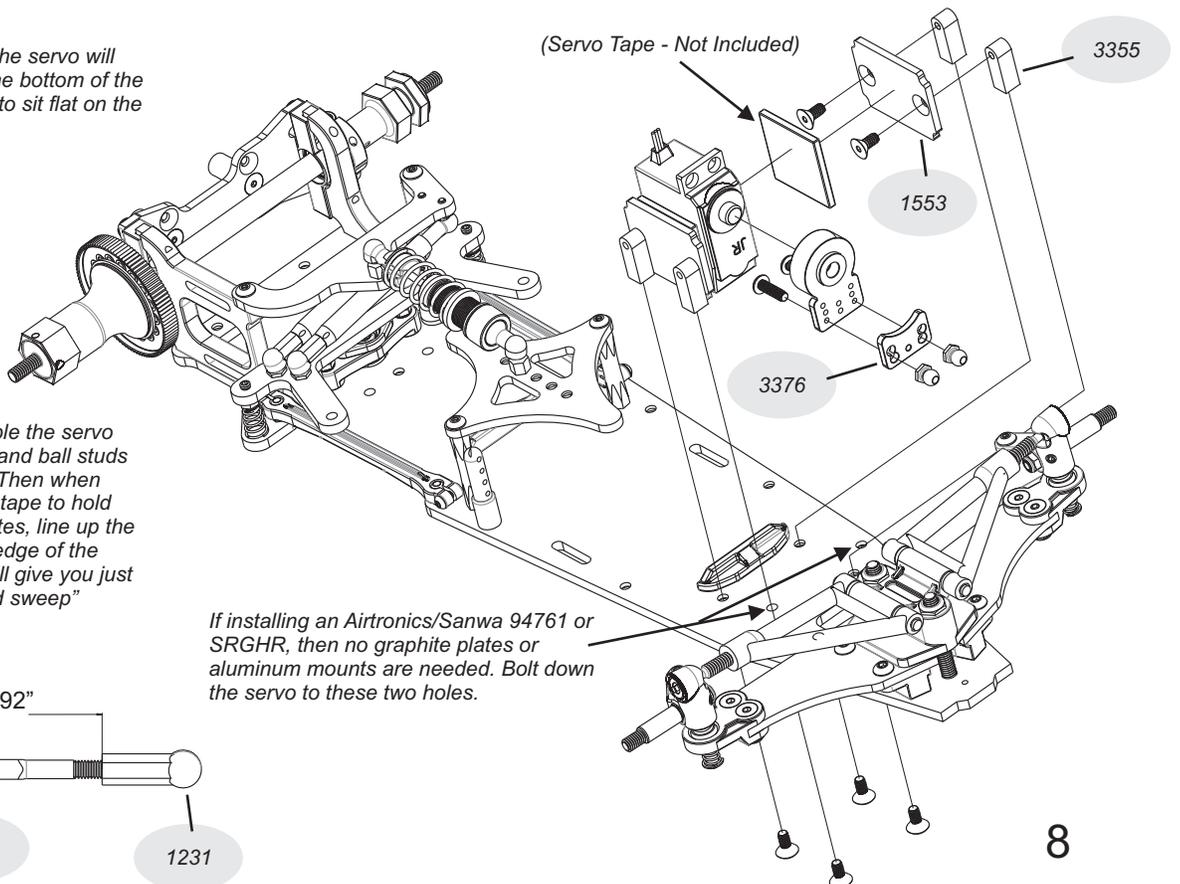
Servo Alignment - Assemble the servo saver, servo saver brace, and ball studs as shown in the diagram. Then when using the two-sided servo tape to hold the servo between the plates, line up the servo case flush with the edge of the graphite plates and this will give you just the right amount of "tie-rod sweep" (steering ackerman).
