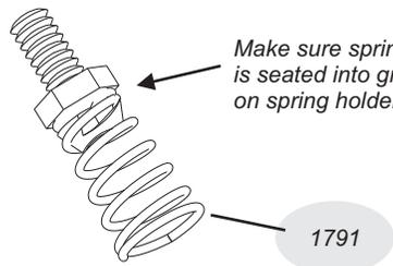
Make sure spring coil is seated into groove on spring holder.
