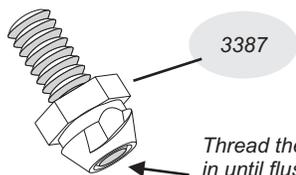
Thread the set screw in until flush with the bottom of the holder.
