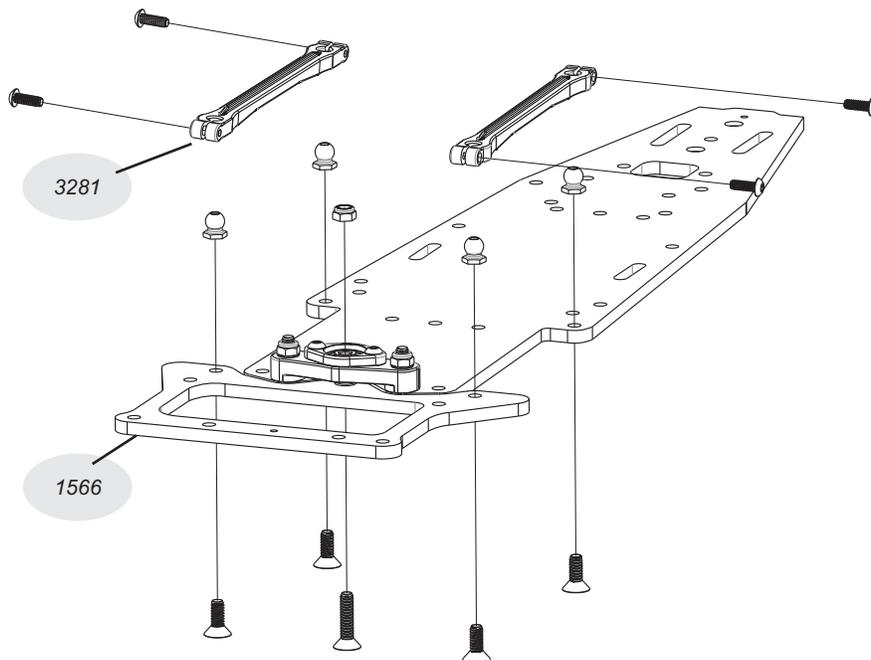
**\*NOTE -** Before installing, inspect the side links and you will notice that the screw holes on one side of the link are larger than the holes on the other side. Before popping the links on the balls, be sure that the larger hole faces toward the outside of the chassis.
