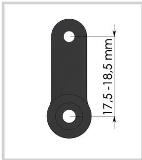
**Note:** Recommended length of servo arm is 17,5-18,5mm. We highly recommend our **P40F** and **P40K** Servo Arms. We also recommend our **AS-701L** Brushless Low-Profile Car Servo. Awesomatix **AS-701L** servo has an integrated servo holder and can be screwed to the chassis directly.
