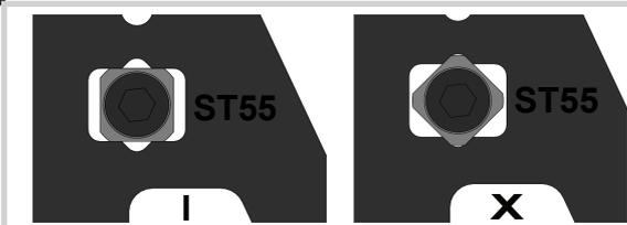
**Note:** Two orientations of **ST55** bushing are possible. Position **I** provides an increased flex of the chassis.
