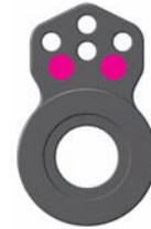
Note the orientation of servo saver when servo is in neutral.
