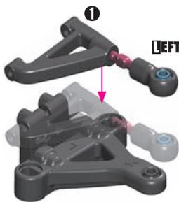
If the arm does not have enough play, remove the clips and thin the clips slightly with sandpaper. The arms must have free movement and not bind.
